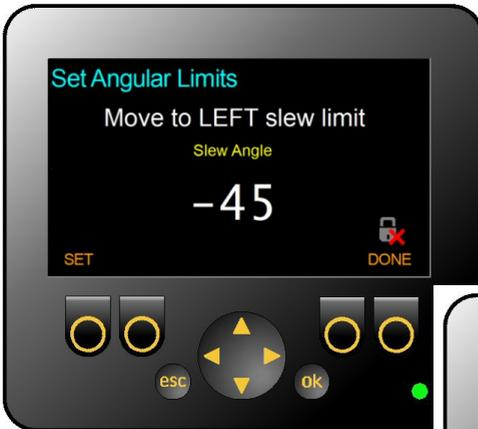
1. Slew to the required left slew limit and press **SET**.
