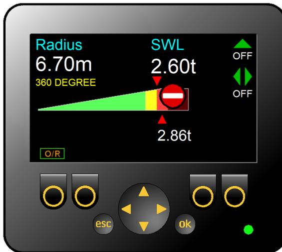
Pushing the **O/R** button will release all the hydraulic controls. The internal and external alarms will continue to sound. The override will automatically clear when the machine becomes safe.
