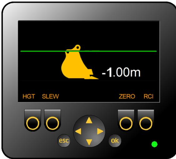
Once the desired depth has been achieved, the system can be re-zeroed at the base of the excavation - now the correct depth will correspond to 0.00m on the screen.
