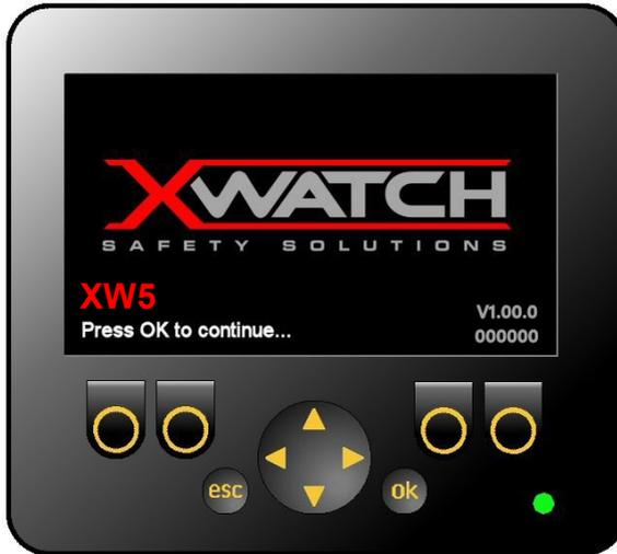
The RCI will start automatically when the machine ignition is switched on. After a short delay, while the system transfers information from the I/O controller, the display above will appear. The RCI will operate after 10 seconds, or immediately if **ok** is pressed. The logo displayed may differ.
