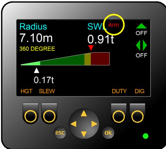
If the safe working load is limited by hydraulic capacity rather than stability, the offending service will be shown next the SWL label. Depending on machine type, this can be:
