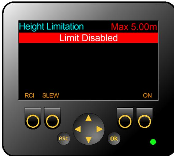
If **OFF** is used from an active height limitation page the display will change as shown above and all motion control will be released. Equipment height is no longer monitored.
