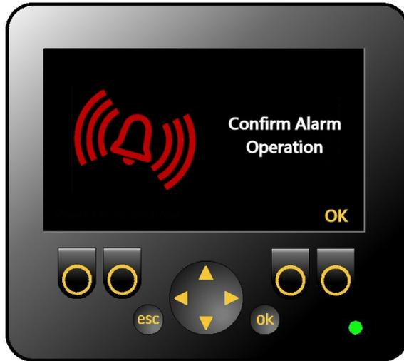
If the XW Series device has an RCI, the page above will be displayed. The internal and external alarm will sound. If the system has hydraulic control, all motion will be inhibited.
