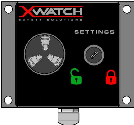
The Settings key switch is an **option** and is mounted inside the machine cab. If fitted, the key must be in the unlocked position to allow the setting of limits and the enable/disable of the operational modes. If the switch is not fitted, all features are available to the operator.
