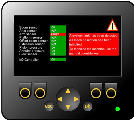
The system continuously monitors the health of the sensors and the IO Controller inputs and outputs. If a problem is detected, the screen shown above will appear. If the system has motion control valves fitted, the system will failsafe and close all the valves. The failed sensor(s) will be shown in red.
