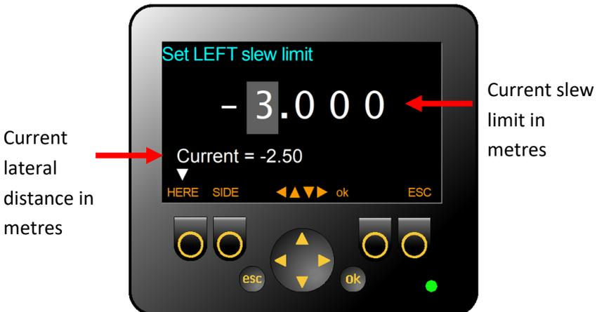
When setting slew walls when the machine is slewed over the rear of the machine, the left limit will actually be on the operators right hand side. This is because the walls are with respect to the undercarriage.
