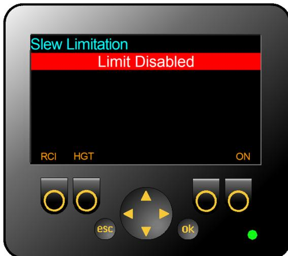
If **OFF** is used from an active slew limitation page the display will change as shown above and all motion control will be released. Equipment slew is no longer monitored.
