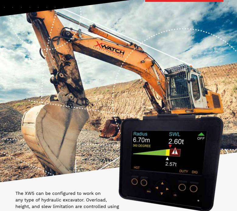
height, and slew limitation are controlled using proportional soft-stop hydraulic valves providing accurate and repeatable performance without detriment to the machine. A basic dig depth monitor is available when the RCI is not required. If hazards arise, XW5 will automatically flip to the relevant display page. Tracked machines have automatic sectored lifting duties for over the front/rear operation and over the side. Load charts are ISO10567 compliant.
