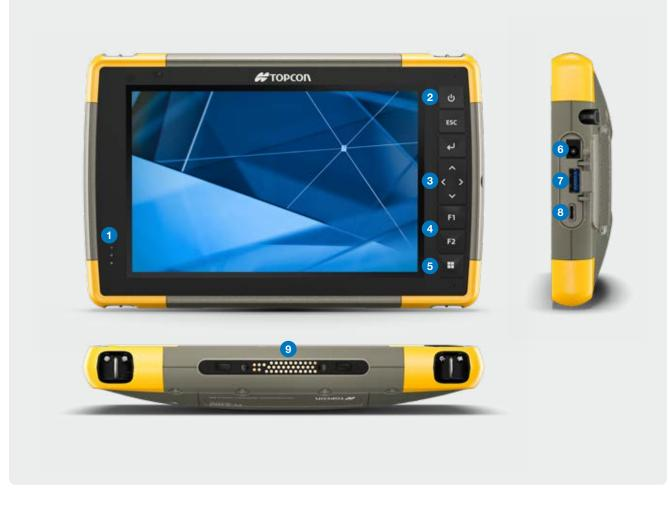
1LED indicators4Customizable function keys7USB type A2Power key5Windows® Start button8USB type C34-Way directional cursor control6Power input9External keyboard contact strip
